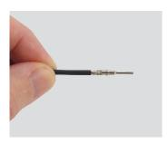
Step 1: Grasp crimped contact approximately one inch behind the contact barrel.
