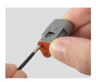
**Step 3:** Hold the rear seal in place, as removing the contact will displace the seal.
