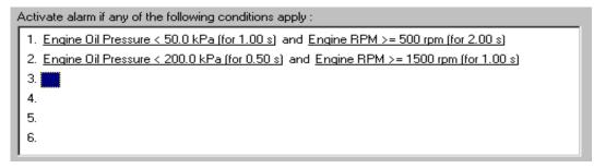
In the case of alarms, the condition can also contain an increment or decrement amount, which may increase or decrease the test value by a certain amount each time the alarm is acknowledged. The number of times this value is incremented can be limited.
