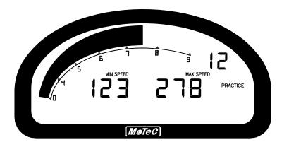
The Practice Display is used to display basic information, plus information to help the driver improve lap times, e.g. Lap Time, Lap Gain / Loss, Maximum Straight Speed, Minimum Corner Speed or Corner Exit Speed.
