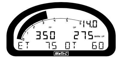
The Warm-up Display is used to display important engine sensor readings during engine warm-up, e.g. RPM, Battery Voltage, Engine Temperature, Oil Pressure, Oil Temperature and Fuel Pressure.
