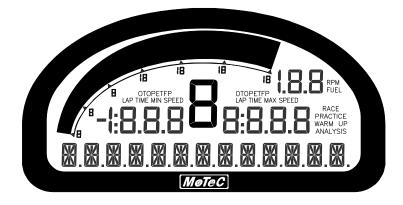
The display has three main modes of operation, Race, Practice and Warm-up. Refer to the Display Modes section for details.
