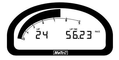
The Race Display is normally used to display minimal information, e.g. RPM, Lap Time, Fuel Remaining or Laps Remaining.
