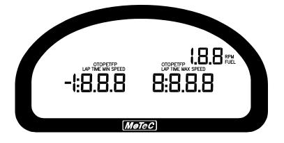
The three Numeric Displays (Left, Right and Top Right) can be programmed to display any value, which may be different for each of the display modes (Race, Practice and Warm-up).
