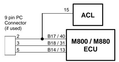
**Note** The data to the ACL will be interrupted while a PC is connected (DOS software only)
