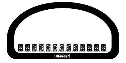
The 13-digit Bottom Alpha / Numeric display can display up to 20 lines of information that can be scrolled up or down using the externally connected buttons. Each of the 20 lines can display up to 3 channel values at a time.
