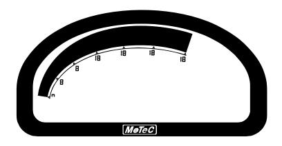
The 70 segment Bar Graph has a user definable range and is typically used as a tacho, however it can be used to display any other value. When used as a tacho it may be configured to show up to 19000 RPM.
