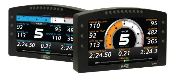
The C187 comes standard as a combined 7" full colour display, powerful control device and fully programmable data logger with 250 MB memory (500 optional). The anti-reflective, high contrast display is clear and vibrant in direct sunlight.
